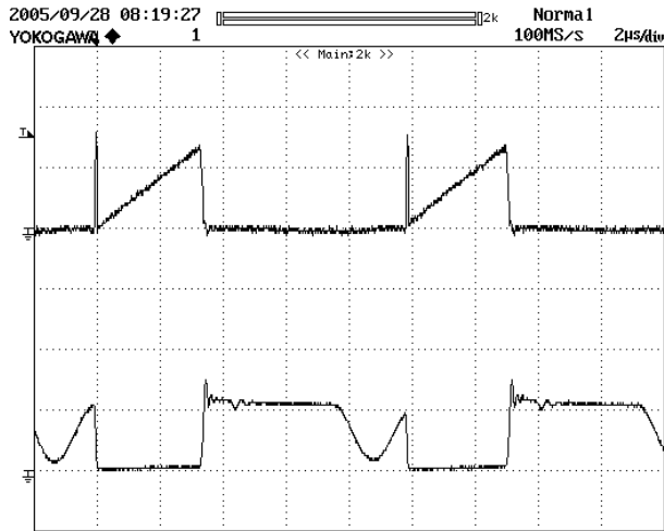
Figure 12 – 90 VAC, Full Load. Upper: I_{DRAIN} , 0.10 A / div. Lower: V_{DRAIN} , 200 V, 2 \mu s / div.
